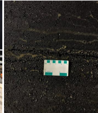
(e) Final texture of low permeability mix
